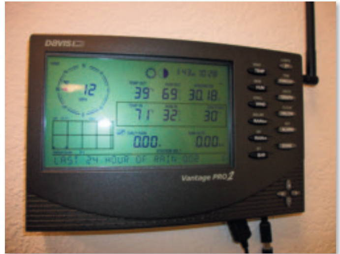
INFORMATION CENTER — The new weather station installed in the AGGRAND growth plots transmits all of the pertinent information to this console and is archived electronically.
